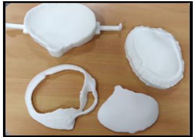
Fig. 4: Cranial mold fabricated through 3D printing with PLA
