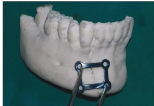
Figure 2: Adaptation of three-dimensional plate to the fracture site preoperatively on the stereolithography model
