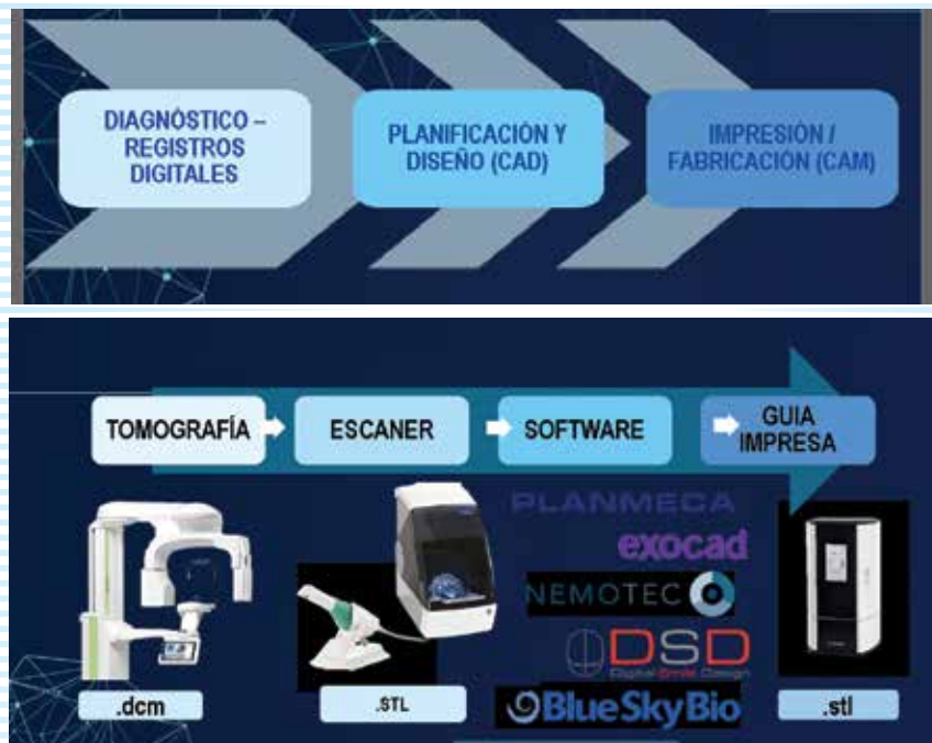
FIG.1 : Digital workflow in dentistry, has as fundamental pillars, the tomographic registration and the scanning that supports the diagnosis, planning (CAD) with design software, and manufacturing (CAM) in 3D printers
