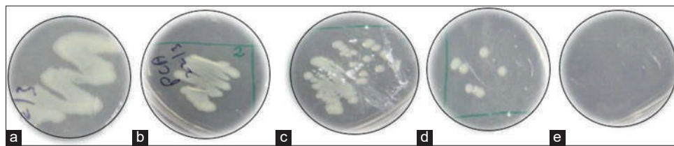
Figure 4: Agar plate counts after different exposure times of plasma; (a) Control plate (no treatment); (b) 2 s; (c) 5 s; (d) 10 s; (e) 15 s
