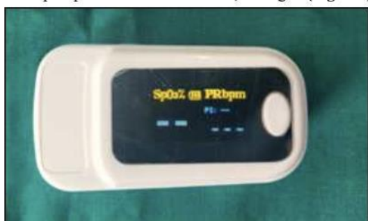
Figure I- Pulse oximeter SpO 2 - Oxygen saturation PRbpm- Pulse rate (beat/minute)
