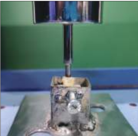
Figure 1: Sample mounted in self-cure acrylic resin subjected to universal testing machine
